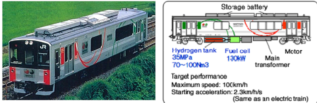
Figure 4.1 NE Train: Fuel Cell Hybrid Train Developed by East Japan Railway Company
