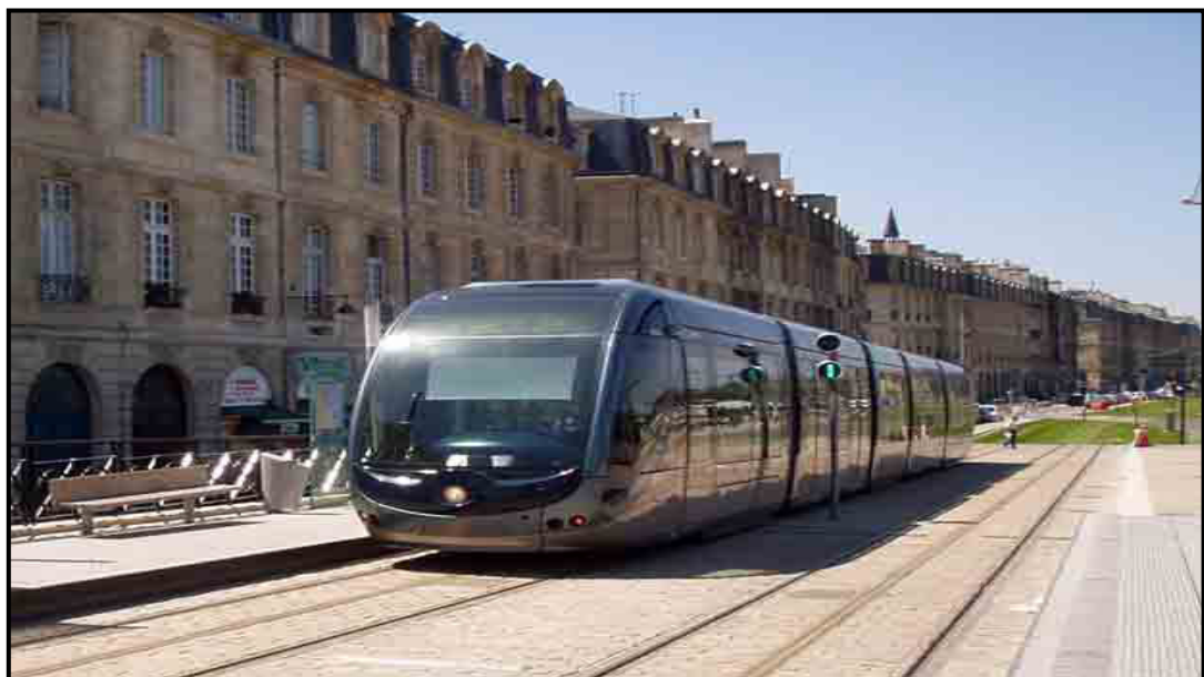
Figure 5.2 Bordeaux LRT with Ground Power Supply located between tracks
