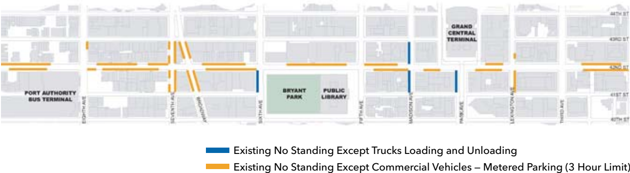
FIG 18. Inventory of existing delivery truck parking locations at the peak midday hours of usage for each curb; the curb feet-minutes occupied were carefully observed and compared with the curb space available.
